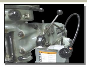
EZ position steel flex arm does not interfere with quill handle operation
