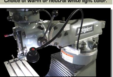
Flexible lighting positioned where you need it with 30 inch length steel flex arm
