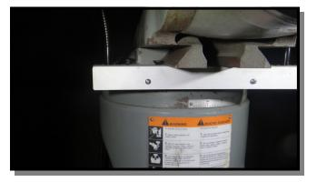
EZ ram dovetail "slide-on" mounting with no holes to drill or tap
